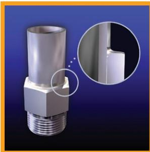
When the parts are up to temperature (typically a dull red color), touch the Handy One flux cored wire to the joint area. The flux and alloy will melt and be drawn by capillary attraction down into the joint. The minimal amount of flux in the Handy One cored wire reduces flux inclusions, yet provides complete alloy penetration and high strength joints.
